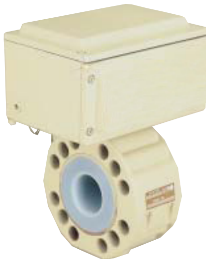
Figure 8: Wafer-type electromagnetic flowmeter is lightweight, compact, and can be easily installed between existing pipe flanges. The no-moving-part instrument has negligible pressure drop and can handle numerous liquids and slurries, provided they are conductive.
