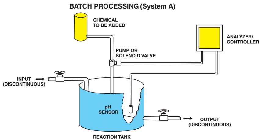
The final control element can be a pump or an ON/OFF valve. Sizing of the final control element is complicated and depends on many factors. This is one situation where a titration curve can be invaluable. In many cases, it may be necessary to use two final control elements, each delivering different amounts of chemical and having different setpoints. For example, one valve may deliver 1 GPM of caustic below 3 pH and another may deliver 0.1 GPM of caustic below 4 pH.
