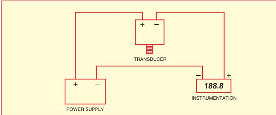
Figure 3: Typical wiring configuration for current output transducer
