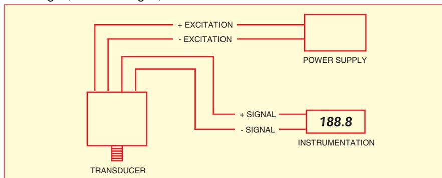
Figure 1: Typical wiring configuration for millivolt output transducer
