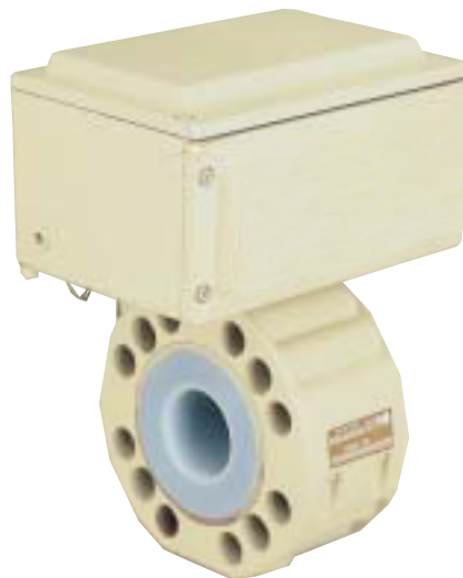
Figure 8: Wafer-type electromagnetic flowmeter is lightweight, compact, and can be easily installed between existing pipe flanges. The no-moving-part instrument has negligible pressure drop and can handle numerous liquids and slurries, provided they are conductive.
